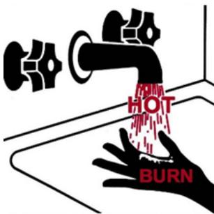
Water temperatures over 125°F (52°C) can cause severe burns or scalding resulting in death.
