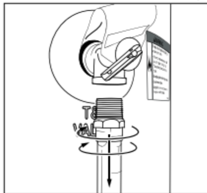
Figure 10 - Removing the T&P Relief Valve discharge pipe.
