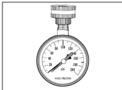
Figure 4 - Use a Water Pressure Gauge to make sure your home's water pressure is not too high.
