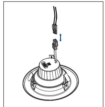
Plug the female connector of the RETROFIT KIT onto the male connector of the QUICK CONNECT ADAPTER.
