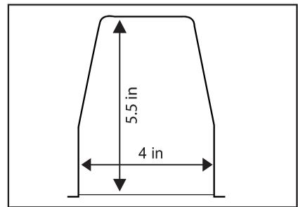
This 4" retrofit kit must be installed in a can with dimensions described within above diagram.
