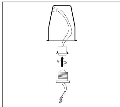
Screw in the E26 quick connect adapter into the recessed can's socket.
