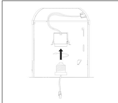
Screw in the E26 quick connect adapter into the recessed can's socket.
