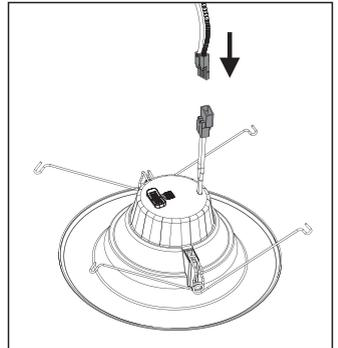
Plug the female connector of the RETROFIT KIT onto the male connector of the QUICK CONNECT ADAPTER. ctor
