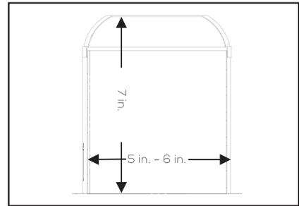
This 5/6" retrofit kit must be installed in a can with dimensions described within above diagram.
