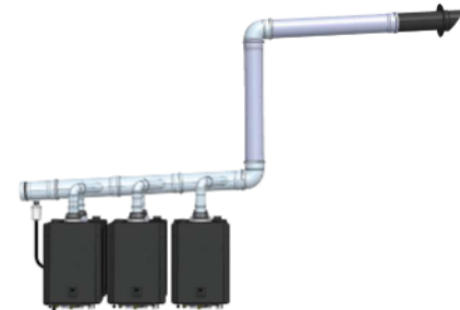
ROOM AIR WITH HORIZONTAL EXHAUST (NEW)
