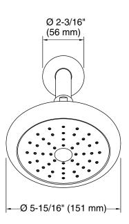
Technical Information All product dimensions are nominal. Showerhead/Body Spray: Rated maximum 1.75 gal/min (6.6 l/min) flow: Pressure: 45 psi (3.1 bar) Notes Install this product in accordance with the installation instructions.
