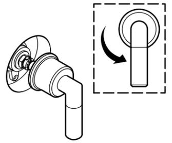
**6** To adjust position, remove the handle and valve stem adapter. Turn the spline adapter.
