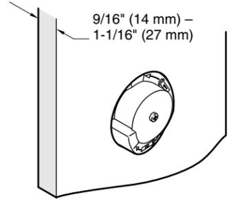
**Thick Wall:** Use the #2 adapter and the 1-3/4" (44 mm) screw.
