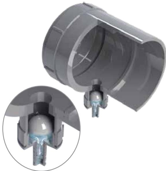
The System 636 Cleanout Condensate Drain is designed to be installed at the end of the exhaust manifold to effectively allow any accumulation of condensate or rain to drain. The Cleanout Condensate Drain is available in sizes ranging from 6" to 12" in both PVC and CPVC.
