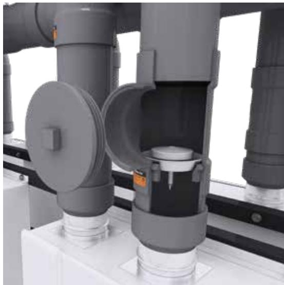
The first engineered Backflow Valve to be certified to the ULC S636 standard, available in 4" in both PVC and CPVC. The backflow valve is designed to be installed on the vertical exhaust vent of each unit to prevent the exhaust flue from flowing back into the unit.
