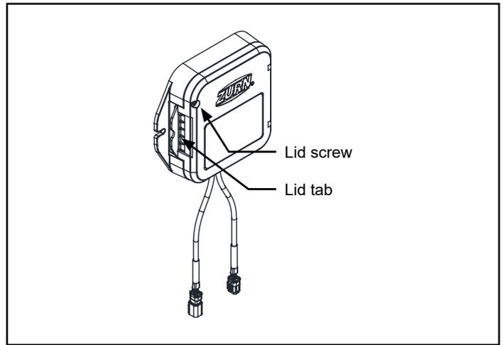
3. Install supplied lithium batteries. Close lid and secure by pressing on the lid tab until it snaps into place. Then tighten lid screw.
