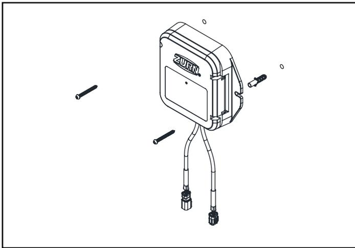
2. Loosen lid screw with supplied 3mm Allen wrench and Open the lid.
