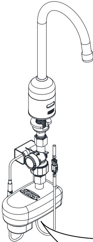
Note: To install Braided Hose, need to hold swivel nut on control box or mixing valve in position then apply torque by hand or wrench to install. Do not over torque the nut.
