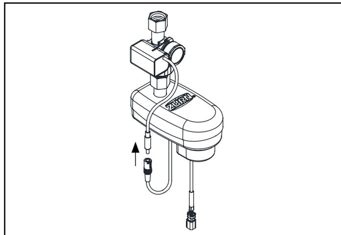
3. Open battery module using supplied Allen wrench and install supplied alkaline batteries in the electronics module in the configuration as shown.
