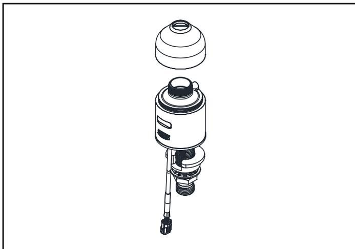
2. Install the spout onto the faucet body by turning the spout nut clockwise. Feed the spout nut cover through the spout back onto the faucet body.
