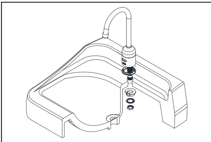
1b. Install spout to sink wall using spout base o-ring, plastic mounting washer, mounting nut, and shank elbow.
