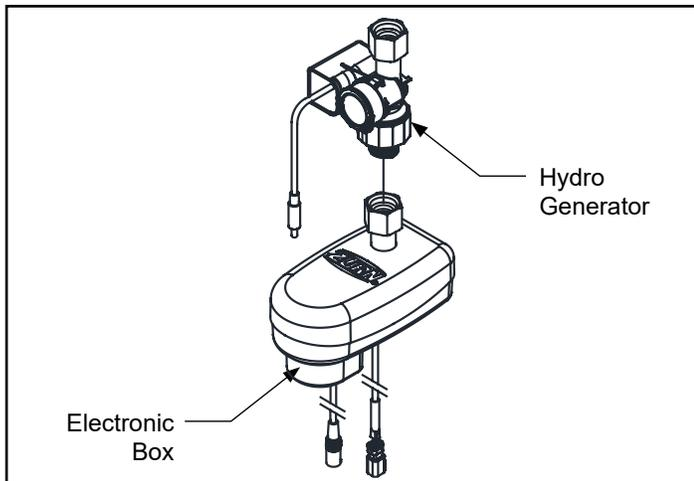
2. Connect electronics module power cable to hydrogenerator.
