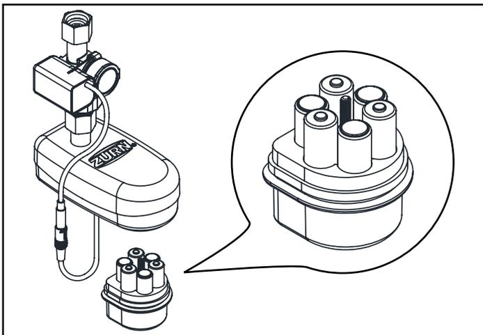
4. Tighten electronics module assembly with hydrogenerator to shank and connect water line(s).
