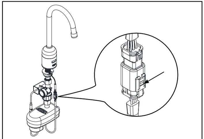
5. Connect the electronic module to the connected monitor first, and the spout to the connected monitor second.
