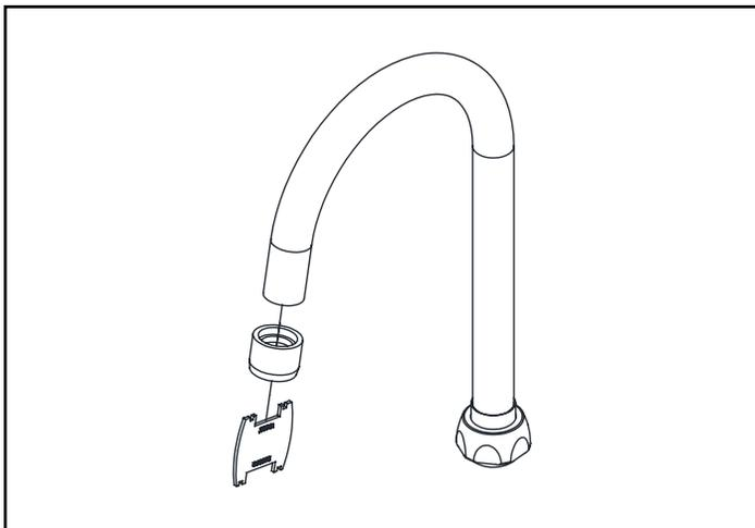
2. Install the spout onto the faucet body by turning the spout nut with a adjustable wrench clockwise.
