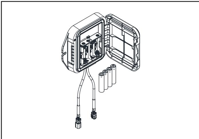
4. Unplug the sensor connection from the spout to the electronic module by compress the clip on the connector and pull apart.
