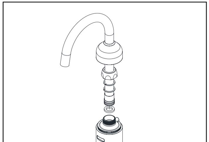
3. Align the small hole on the spout nut cover to the set screw to the back of the faucet body. Use the provided hex key wrench to lock the spout nut cover in place by turning in it clockwise.
