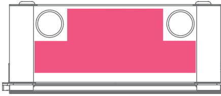
Top, surface-mount: Myers hub recommended outdoors
