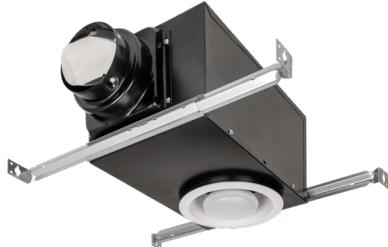
With an energy-efficient motor, the bathfan Recessed RCS80L provides 80 CFM (38 L/s) @ 0.1 in. wg. (25 Pa) of airflow alongside quiet operation. The recessed ENERGY STAR® approved light provides a sleek yet aesthetically pleasing look, especially for rooms with low ceilings. The exhaust fan comes with four (4) adjustable hanger bar mounting brackets that extend up to 24 in. (610mm).
