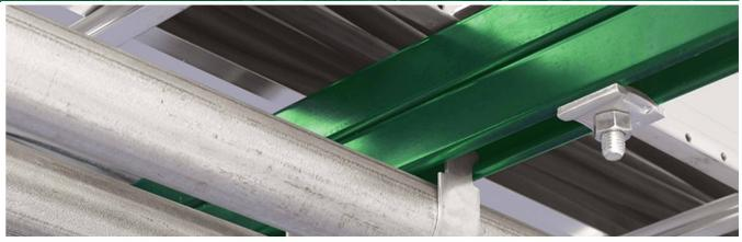
H-Strut Channels are manufactured by a series of forming dies and rolls which progressively work the strip seal into the desired channel configuration. This method produces a cross section of uniform dimensions within a tolerance of plus or minus 0.015", on outside dimensions.
