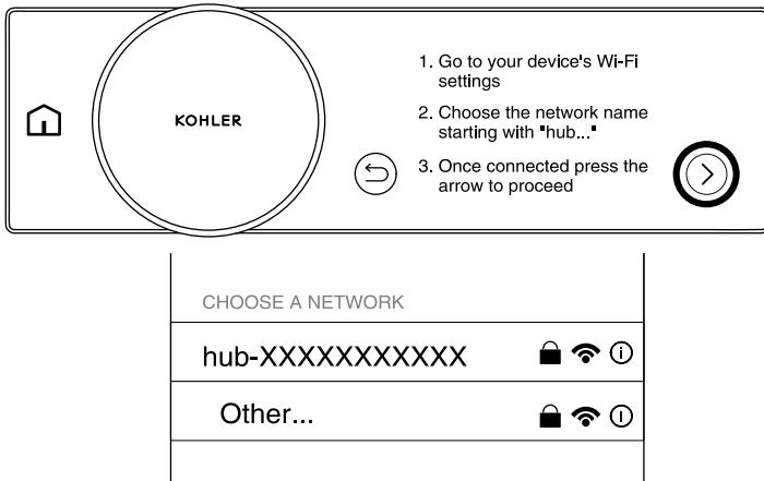
**NOTE:** The system controller is now in access point mode and discoverable by your device's Wi-Fi settings. If no action is taken for 30 minutes, the system controller will no longer be in access point mode. Press the back button and then press the arrow to return the system controller to access point mode.
