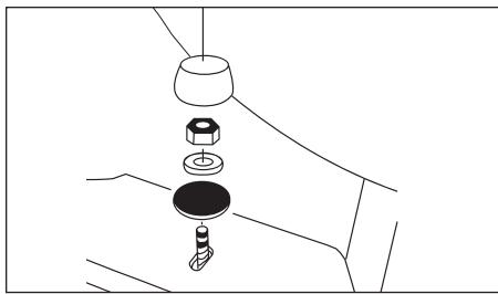
7. Install the washers, nuts and caps on the flange bolts snugly. Be careful not to overtighten because the china may break.
