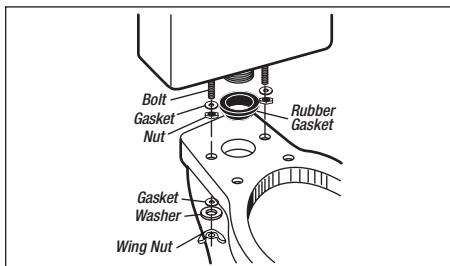
8. Install tank-to-bowl gasket and tank bolts with provided gaskets, washers and nuts. Then, attach tank to bowl by placing gasket, washer and wing nut onto each protruding bolt.
