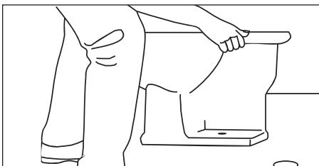
5. Gently lower the bowl onto the flange, making sure the flange bolts protrude through the toilet bolt openings.
