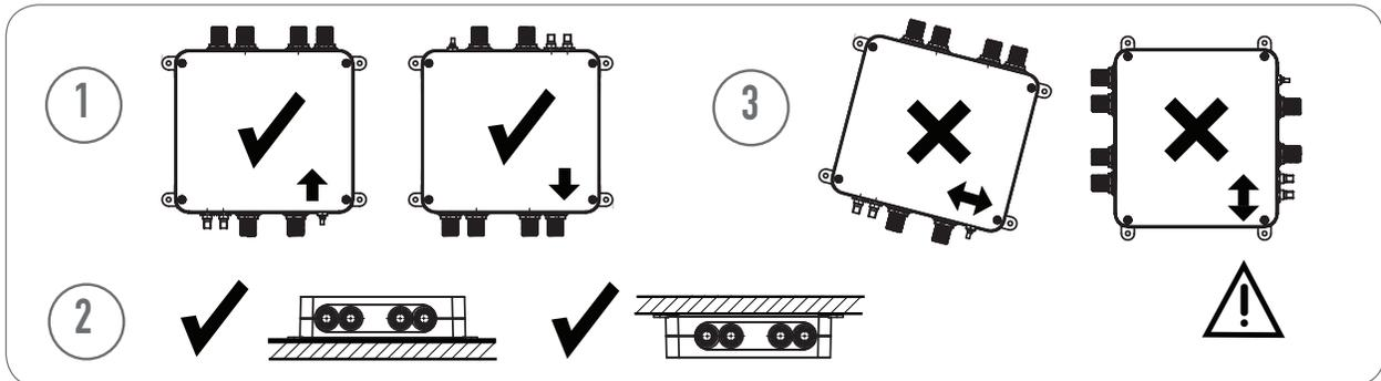
1. Mounting on a vertical or horizontal surface with inlets pointing up or down/front or back.
