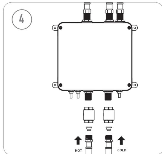
Install filters and connect supply lines. Supply pressure must be at least 20 psi and not exceed 73 psi. The recommended pressure is 43 psi, install pressure reducing valves as required.
