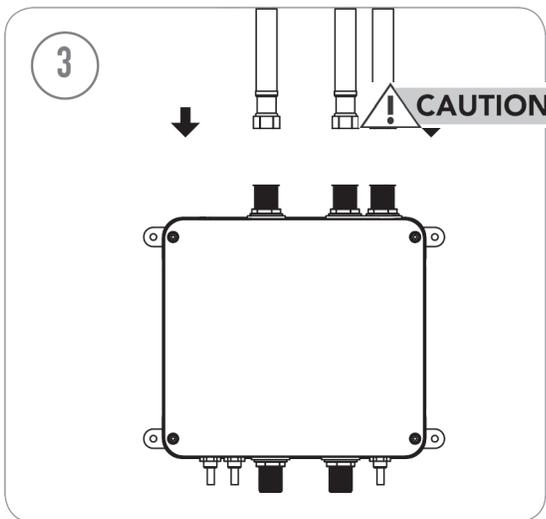
Connect outlet plumbing to the valve. No valves or diverters shall be installed between the valve and the in-shower fixtures. Output 1 must always be plumbed.
