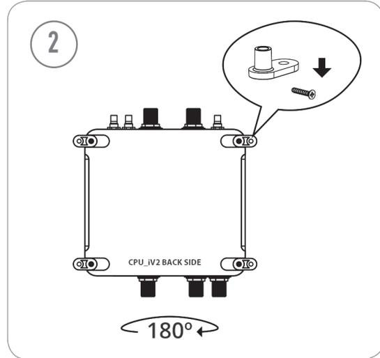
Rotate the mounting feet to the deployed position and attach the valve to the wall using the appropriate screws.
