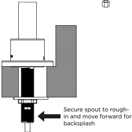
For uneven or porous surfaces use plumbers putty or silicone
