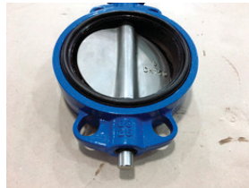
5. Insert the lower stem into the disc by pushing the valve body and disc assembly down onto the stem. Then tap the lower stem further in beneath the internal threads in the body.
