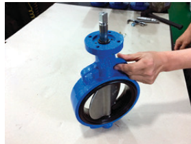
8. With lubricant, insert the upper stem almost all the way into the body. Make sure the stem flats are aligned with the receiving hole in the disc.
