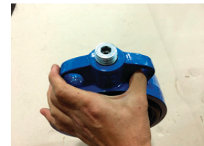
12. Insert the lower stem plug by first applying pipe dope such as Loctite® or an equivalent product to secure the plug.
