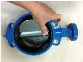
4. Insert the bottom of the disc into the seat over the lower stem. With the disc in the partially open position, push or tap the top of the disc to align with the upper stem hole.
