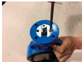
11. With a rubber mallet, tap the upper stem the remainder of the way into the stem. Secure the retainer plate with flat head counter-sunk screws.
