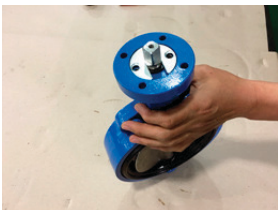
10. Slide the retaining plate onto the groove located just below the square drive of the stem. Align the screw holes with the holes in the body's top flange.
