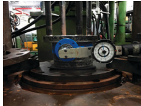
14. If facilities are available, test the valve for torque and shutoff.
