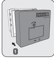
Reinstall the control box cover and secure it with the #2 Phillips screw.
