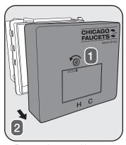
Remove the control box cover by using a #2 Phillips screwdriver to loosen the cover screw.
