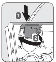
Be sure to seat the hose firmly before reinstalling the metal key and securing it with the yellow locking tab.
