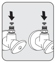
1. Insert the filter screen gaskets into the supply stops.
