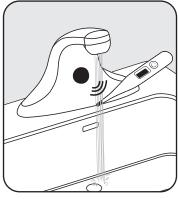
b. Mixed water temperature must be checked at the point of use and the CFC mixing valve adjusted to ensure delivery of water at a safe temperature no exceeding 110°F (43°C). Water temperatures in excess 110°F (43°C) are dangerous and may cause scalding, severe injury or death!
