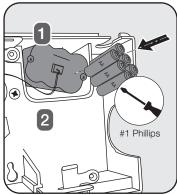
i. Open the yellow battery housing and insert 4 'AA' batteries according to the diagram inside the housing. NOTE: Make sure the batteries are oriented properly before testing the faucet.
