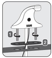
Attach the threaded rods to the bottom of the faucet. Position the gasket accordingly on the sink and lower faucet.
