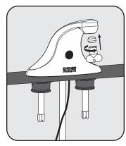
After completing control box install, flush lines completely. Then install outlet cache using provided installation key.
