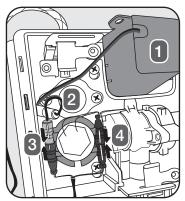
i. Insert LTPS into upper compartment of box, aligning slots with compartment ribs. Attach LTPS adapter wiring connectors (green to green). First green to green, then gray to gray. Note: the connectors are keyed for proper installation.
