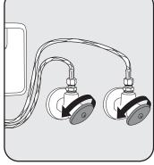
Open the supply stops and check for leaks. Note: water may run through spout.
