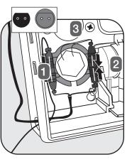
ii. Attach the wiring connectors (gray to gray, black to black). Note: Connectors are keyed for proper installation as shown. Snap completed connections, into the wiring harness as shown.
