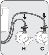
2. Attach the 3/8" female compression supply hoses from the control box to the supply stops. Use a wrench to tighten the nuts to the supply stops.
