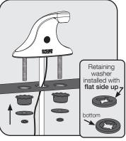
Below the sink, place the basin washer, flat washer and retaining washer onto threaded rod and push secure. Retaining washer will hold in place while securing nut.
