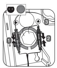
ii. Attach the wiring connectors (gray to gray, black to black). Note: Connectors are keyed for proper installation as shown. Snap completed connections, into the wiring harness as shown.
