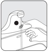
Once wiring is complete, the red sensor light at the faucet outlet will glow continuously for 5 seconds. After the light switches off, place your hands in front of the faucet. The faucet should activate and water should flow.
