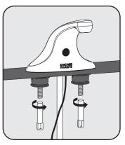
Tighten nut onto threaded rod using a screwdriver, wrench, or 1/2" socket.
