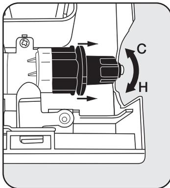
b. Cap must be partially pulled from the valve to adjust temperature. Turn the handle clockwise to decrease temperature or counter-clockwise to increase temperature.
