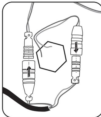
2. Attach power connections as shown in the following sections.
