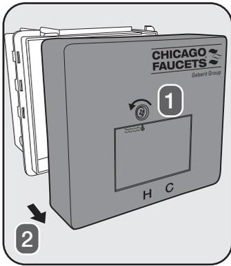
1. Remove the control box cover by using a #2 Phillips screwdriver to loosen the cover screw.
