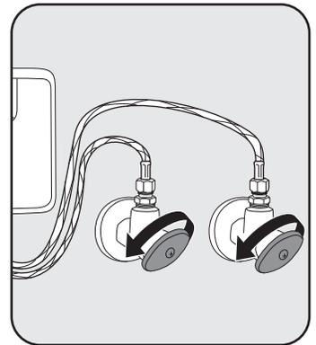
3. Open the supply stops and check for leaks. Note: water may run through spout.
