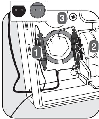
ii. Attach the wiring connectors (gray to gray, black to black). Note: Connectors are keyed for proper installation as shown. Snap completed connections, into the wiring harness as shown.
