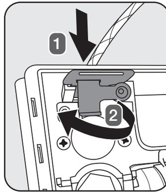
3. Be sure to seat the hose firmly before reinstalling the metal key and securing it with the yellow locking tab.
