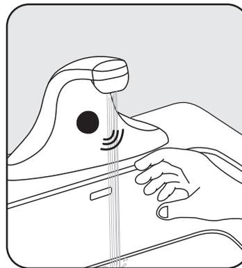
1. Once wiring is complete, the red sensor light at the faucet outlet will glow continuously for 5 seconds. After the light switches off, place your hands in front of the faucet. The faucet should activate and water should flow.
