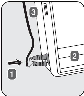
1. Bring wire into box. Use length of box for measurement. Snap into holder on side.
