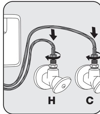
2. Attach the 3/8" female compression supply hoses from the control box to the supply stops. Use a wrench to tighten the nuts to the supply stops.
