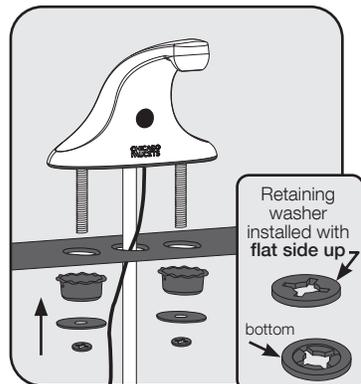
2. Below the sink, place the basin washer, flat washer and retaining washer onto threaded rod and push secure. Retaining washer will hold in place while securing nut.
