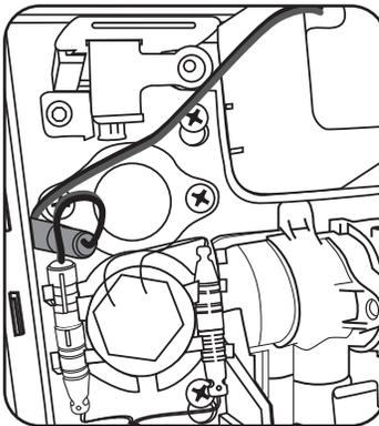
ii. Connect wiring connectors, first gray to gray, then black to black. (Note: the connectors are keyed for proper installation) Snap the completed connections, into the wiring harness as shown. Tuck the completed green connection into the space as shown.
