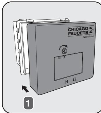
3. Reinstall the control box cover and secure it with the #2 Phillips screw.
