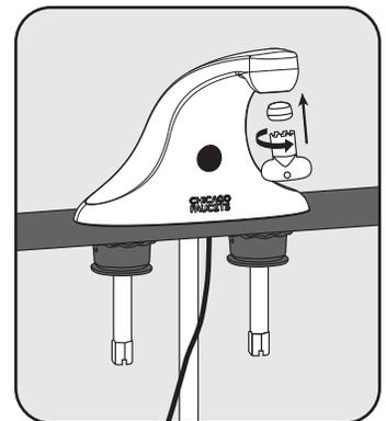
4. After completing control box install, flush lines completely. Then install outlet cache using provided installation key.
