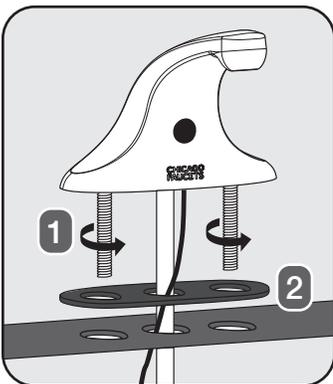
1. Attach the threaded rods to the bottom of the faucet. Position the gasket accordingly on the sink and lower faucet.
