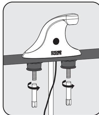
3. Tighten nut onto threaded rod using a screwdriver, wrench, or 1/2" socket.
