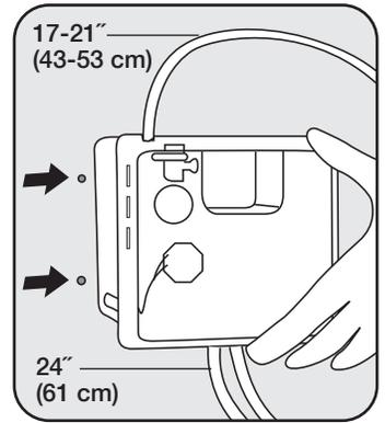
4. Determine the position of the control box under the sink. Hold the control box against the wall and mark the locations of the two mounting holes. Orientation is not critical.
