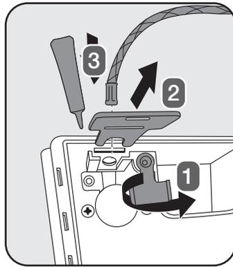
2. Pivot the yellow locking tab and remove the metal key at the top of the control box. Apply silicone-based lubricant to the end of the spout hose and insert it through the hole.
