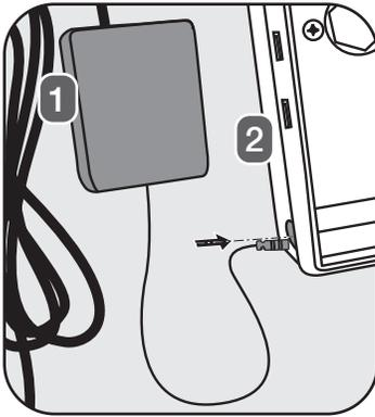
i. Choose a location and mount the transformer. Run the cable from the transformer through the opening in the control box.
