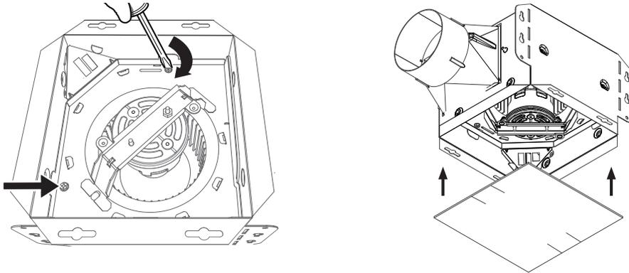
**8** Install the grille trim with screws from parts bag.
