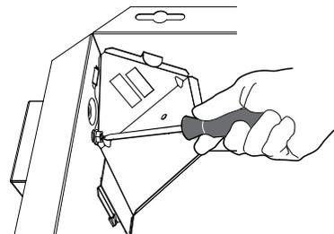
**7** Install the blower assembly with provided screws. Plug in blower.
