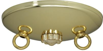
**90-194** - Bath Swag Canopy Kit; Brass Finish; 5" Diameter; 3- 7/16" Holes; Includes Hardware; 10lbs Max
