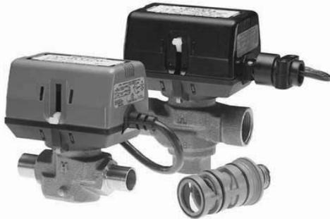
These 2-position (open/close) control actuators are used with VCZ1000, 1100, 6000 and 6100 series hydronic valves in a normal indoor environment to provide quick opening/closing to control the flow of hot and/or chilled water or glycol solution to 60% concentration. They are designed for on-off "zone" control of heating/cooling systems, or to control individual fan coil, baseboard radiator or convector applications.
