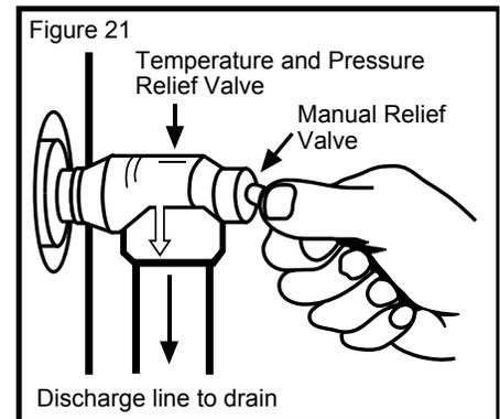
at an adequate drain. Standing clear of the outlet (discharged water may be hot), slowly lift and release the lever handle on the temperature and pressure relief valve to allow the valve to operate freely and return to its closed position. If the valve fails to completely reset and continues to release water, immediately shut off the manual gas control valve and the cold water inlet valve and call a qualified person.
