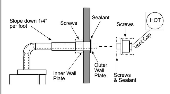
9. Position and fasten the inner wall plate to the inside wall using an appropriate fastener for the specific wall construction. Apply silicone sealant between the inner wall plate and the inside wall.
