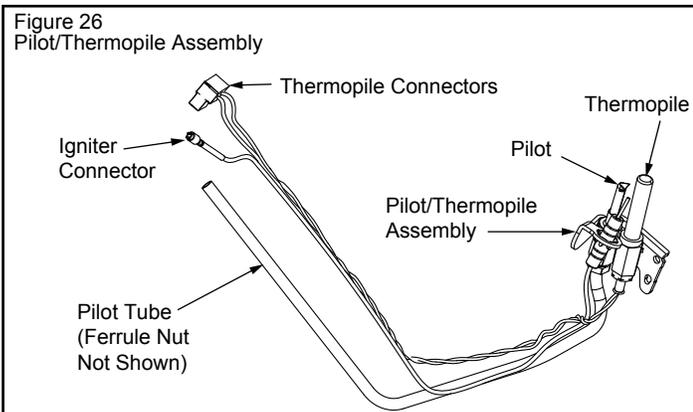
7. Reconnect the pilot tube and tighten the nut securing it to the pilot assembly. To prevent any bending of the pilot bracket, use pliers to hold the pilot assembly bracket while tightening the pilot nut.
