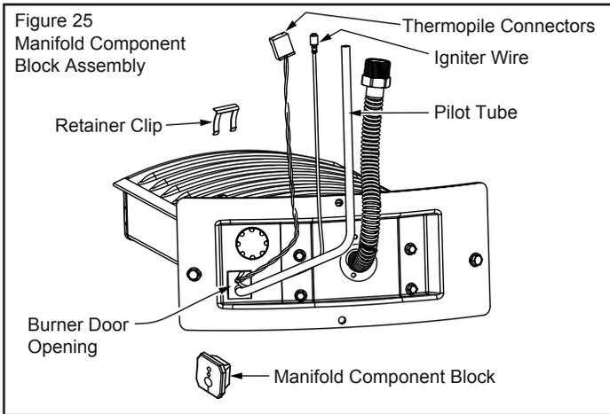
3. Locate and remove the phillips screw attaching the pilot to the pilot bracket, then pull the pilot/thermopile assembly (including the igniter wire) out of the burner door assembly.
