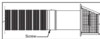
Figure 8 - Completed Vent Connection
