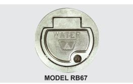
Exterior Finish: Box & Door - Chrome (CH) Only Designed especially for tilt-up wall construction. Install through 6" diameter hole. Two 3/8"-16 tapped holes for all-thread anchors in back of box. Lift and latch door stays open when hydrant is in use.
