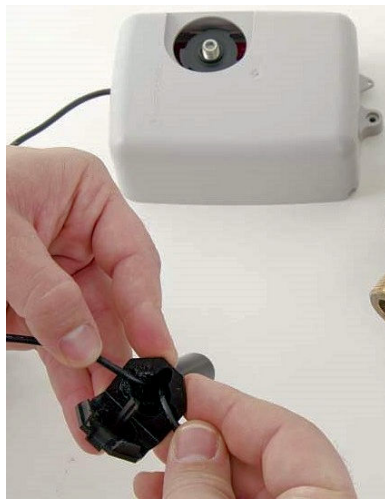
Figure 11 – Gray Wires in Slot
