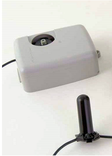
Figure 12 – Cover in Place
