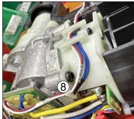
(8) Place solenoid and work light wires into motor housing ribs.
