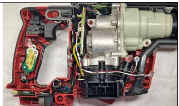
(11) Tuck hall board wires into housing ribs.
