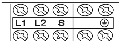
Fig. 17 —Control and Power Wiring on Indoor Unit
