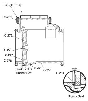
C-250 Cover - Cast Iron ASTM A126 CL.B
