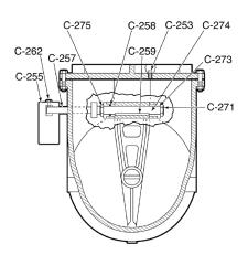
2"-12" Swing Type Lever and Spring Check Valve Parts
