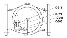
C-305 Hinge Plug – Brass ASTM B21
