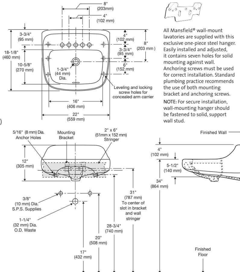
All Mansfield® wall-mount lavatories are supplied with this exclusive one-piece steel hanger. Easily installed and adjusted, it contains seven holes for solid mounting against wall. Anchoring screws must be used for correct installation. Standard plumbing practice recommends the use of both mounting bracket and anchoring screws. **NOTE:** For secure installation, wall-mounting hanger should be fastened to solid, support wall stud.
