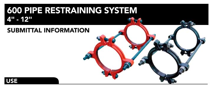
The Series 600 is a multi-purpose pipe restraint system for PVC and ductile iron pipe joints. Configurations are available for use on bell and spigot joints, push-on fittings with restraint ears, mechanical joints, Romac Style 501 and 511 flex couplings. They are engineered to eliminate the need for thrust blocks or other methods of restraint. Not for use on polyethelene pipe, plain end mechanical joint fittings or steel pipe.
