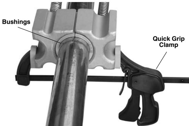
Figure 4 – Attaching Freeze Heads Using Quick Grip Clamp
