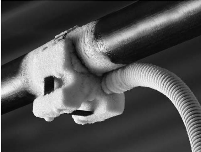
Figure 9 – Freeze Head Frozen to Pipe
