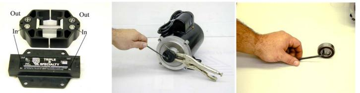
It is not often needed but should you need to replace the C Kit (cam & bearing) use a set of pliers to hold the shaft behind the bearing and use an Allen Wrench to remove the bearing. Any time you take the pump apart you should lubricate the C Kit (cam & bearing) even if it is not replaced. We recommend a high temperature White Lithium Grease. Once all kits have been either serviced or replaced reassemble the test pump in the reverse order it was disassembled.
