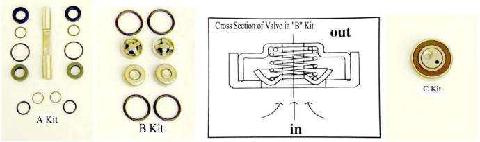
Pictured above are the three Kits (A,B, & C) that are needed to rebuild the pump end of the HT-89A or the HT-90E Test Pumps. The procedure for rebuilding the Tru-Test 120 volt & 12 volt D/C is basically the same as the above, however the A, B, & C Kits are a different size. You will need to specify which pump you are ordering parts for when placing an order.
