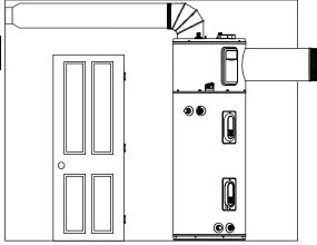
NOTE: Heat pump water heater will operate in rooms less than 700 ft3 down to 450 ft3 but at reduced energy efficiency and reduced performance output. Reduced energy efficiency and performance has not been evaluated by Rheem Manufacturing and not recommended for optimal performance of the unit. When unit is operated in a small enclosure, a door or wall with a minimum of 2.3 sq ft of louvers is recommended to provide proper air changes for unit function.
