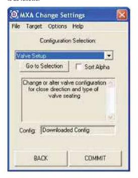
In the *Configuration Selection*, the end user has the option to change the following parameters [COMMIT button saves the desired changes]:
