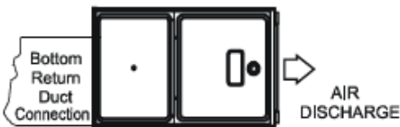
UPFLOW HORIZONTAL RIGHT AIR DISCHARGE
