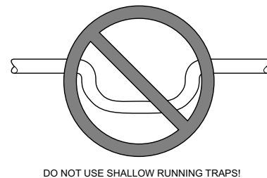
Fig. 12 – Recommended Condensate Trap
