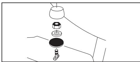
7. Install the washers, nuts and caps on the flange bolts snug. Be careful not to overtighten because the china may break.
