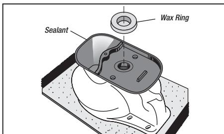
3. Turn the bowl upside down and place it on the flattened carton box to prevent damage.
