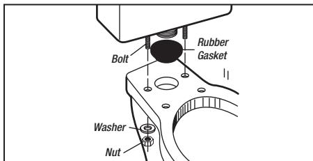
8. Install the tank-to-bowl gasket, tank bolts with washer if it is not already installed, and place tank on bowl.
