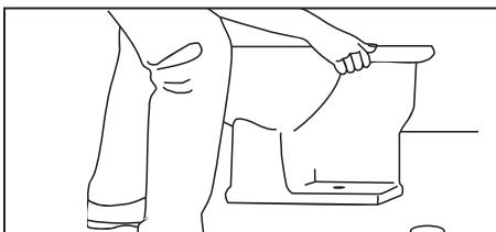
5. Gently lower the bowl onto the flange making sure the flange bolts protrude through the toilet bolt openings.
