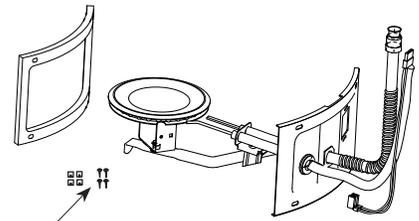
The kit provides extra speed clips and tamper resistant screws.
