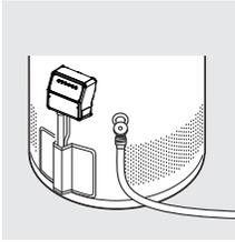
**▲CAUTION:** Shut off gas to the water heater at the manual gas shut-off valve before draining water.
