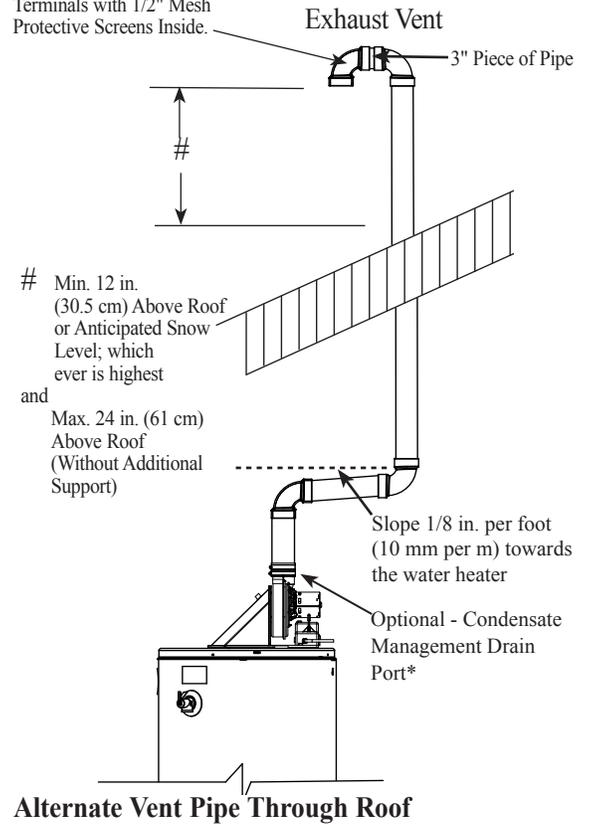
**Alternate Vent Pipe Through Roof**
