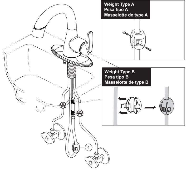
Attach the zinc weight (4) to the hose assembly in the approximate area shown. The weight should be on the upward swing of the hose, toward the spray head in order to provide proper pull to the hose. If further retraction is desired add a second weight.
