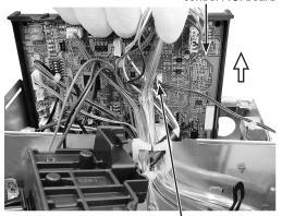
Connector of the refrigerant sensor (CN147)
