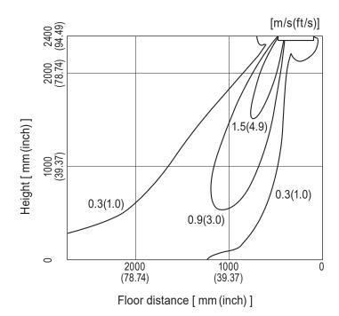
Note: These figures show typical airflow distributions in the conditions above. In the actual installation, they may differ from these figures under the influence of air temperature conditions, ceiling height, cooling/heating load,obstacles,etc.
