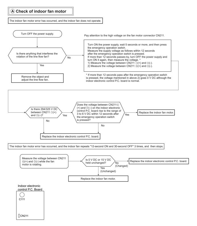
Indoor unit operates by pressing the emergency operation switch, but does not operate with the remote controller.
