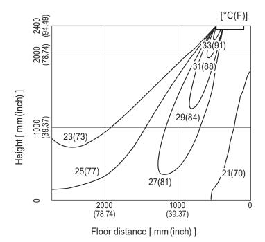
Note: These figures show typical airflow distributions in the conditions above. In the actual installation, they may differ from these figures under the influence of air temperature conditions, ceiling height, cooling/heating load,obstacles,etc.
