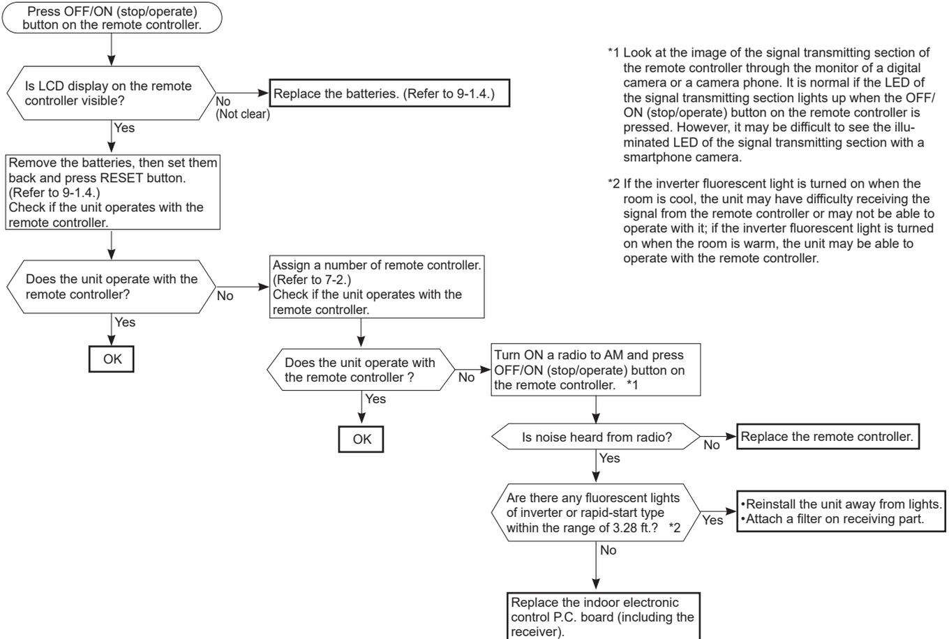
\*1 Look at the image of the signal transmitting section of the remote controller through the monitor of a digital camera or a camera phone. It is normal if the LED of the signal transmitting section lights up when the OFF/ON (stop/operate) button on the remote controller is pressed. However, it may be difficult to see the illuminated LED of the signal transmitting section with a smartphone camera.
