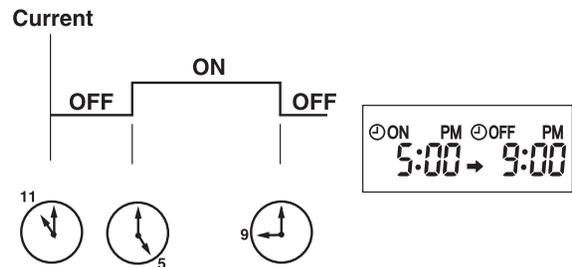
**NOTE:** If the main power is turned OFF or a power failure occurs while ON/OFF timer is active, the timer setting is cancelled. As these models are equipped with an auto restart function, the air conditioner starts operating with timer cancelled when power is restored.
