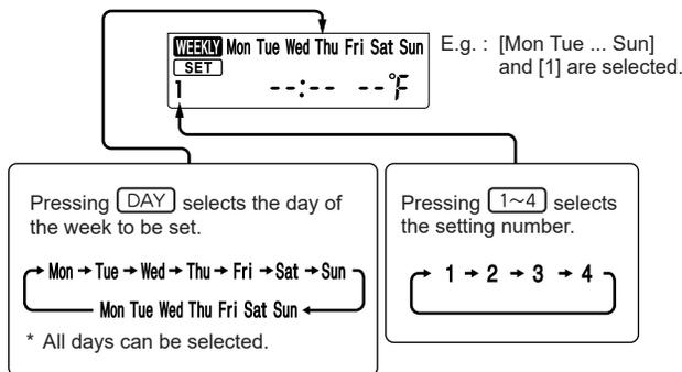
(3) Press **ON/OFF**, **TIME**, and **TEMP** buttons to set ON/OFF, time, and temperature.
