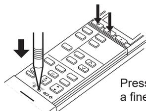
Press RESET button gently using a fine-tipped object.
