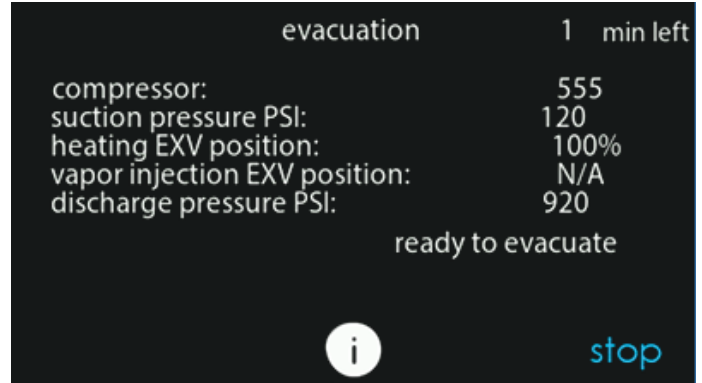
Fig. 28 – Evacuation Status Screen
