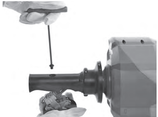
Figure 16A – Removing AUTOFEED Mechanism
