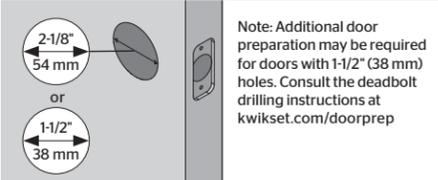
**D** Measure to confirm that the backset is either 2-3/8" or 2-3/4" (60 or 70 mm).
