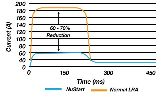
**NuStart is designed for modern scroll compressor technologies in the HVAC/R market – single stage, dual stage, and digital type scroll compressor types. Do NOT use NuStart for inverter type scroll compressors. For other compressor types, contact Nu-Calgon.**
