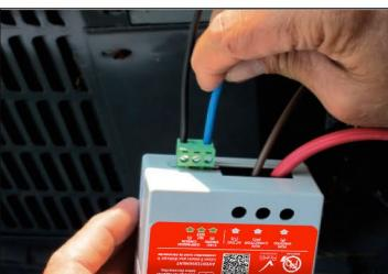
10. Attach the blue wire (supplied) to the Start Winding on the NuStart green terminal connector.
