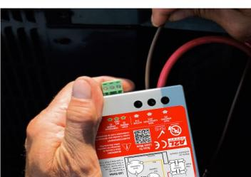
6. Attach the brown wire supplied with the NuStart to the Run Capacitor terminal of NuStart.
