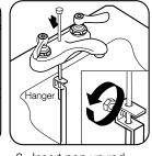
8. Insert pop up rod through holes in hanger and hand tighten.
