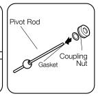
5. Insert pivot ball rod assembly through pivot rod gasket and coupling nut.
