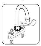
2. Hand tighten sleeve until flush with body.
