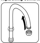
Remove outlet and assemble spout nut over outlet end, until it rests on shoulder of spout joint.
