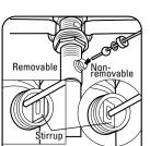
6. Attach pivot rod assembly to body shank.
