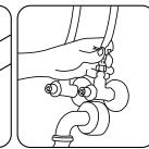
5. Attach hoses or tubes to supply stops. Make sure gasket is installed.
