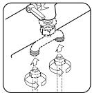
3. Attach supply lines with coupling nuts. Tighten securely.
