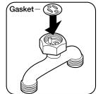
1. Install tee gasket over guide pins and secure coupling nut of tee to body shank.
