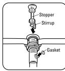
4. Place stopper into body shank cavity orienting the stirrup for removable or non-removable stopper as desired. (see #6)
