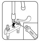
1. Apply Loctite 680, Permabond HH-040 anaerobic sealant, or equivalent NSF 61 approved sealant to threads of spout and tighten spout into base. Back off as necessary for centered position.
