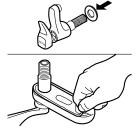
1. Apply putty or rubber washer to underside of faucet body to assure a good seal and level fit.
