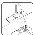
4. Remove outlet and flush lines for about one minute. Replace outlet.
