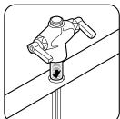
4. Place shank through hole in sink and assemble mounting hardware.
