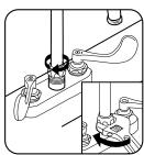
Insert spout assembly firmly into spout base and tighten spout nut.
