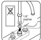
For Rigid Spouts Only 2b. Place 1/8" thick plastic washer into spout base bore and discard plastic split washers.
