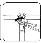
3. Position body shank toward the lift rod. Tighten lock nut until properly sealed.
