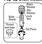
body shank with thread seal tape. Assemble lock nut, slip washer, and basin washer to body shank.
