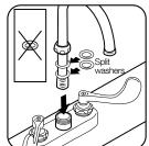
For Swing Spouts 2a. Assemble two plastic split washers to spout joint and discard 1/8" thick plastic washer.
