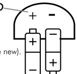
Ensure the batteries are installed correctly. A light to the left of the power button will flash any time a button is pressed. If it does not, reinstall the batteries correctly or check the condition of the batteries.
